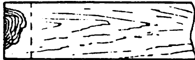
Knots that interfere with nailing should be cut off at dotted line.
